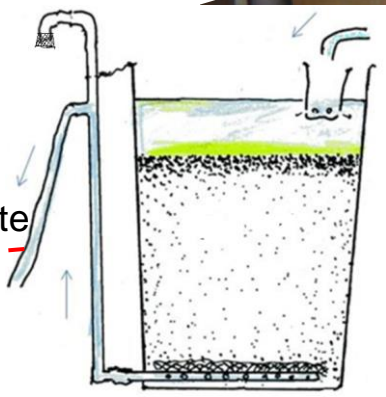
Under drainage porous pipe covered with mesh cloth.
