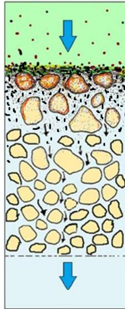
Mechanical filtration by fine sand
