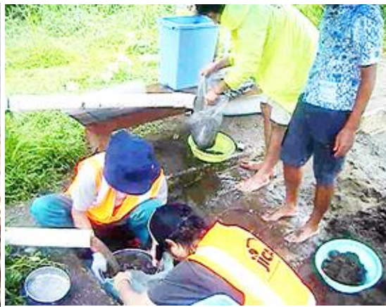
Sand washed and separated with mosquito mesh (1-2 mm)
