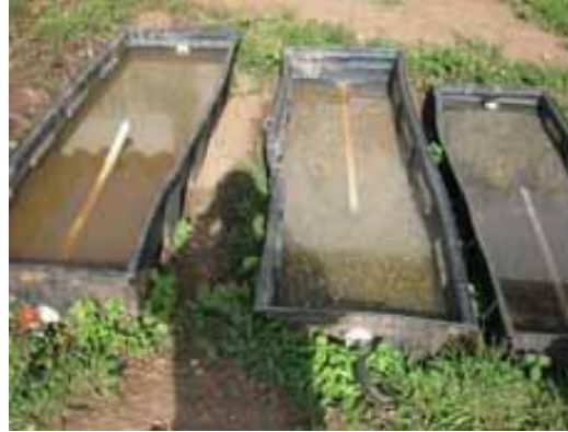
3 steps of gravel filters
