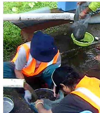
Washing beach sand using mosquito net
